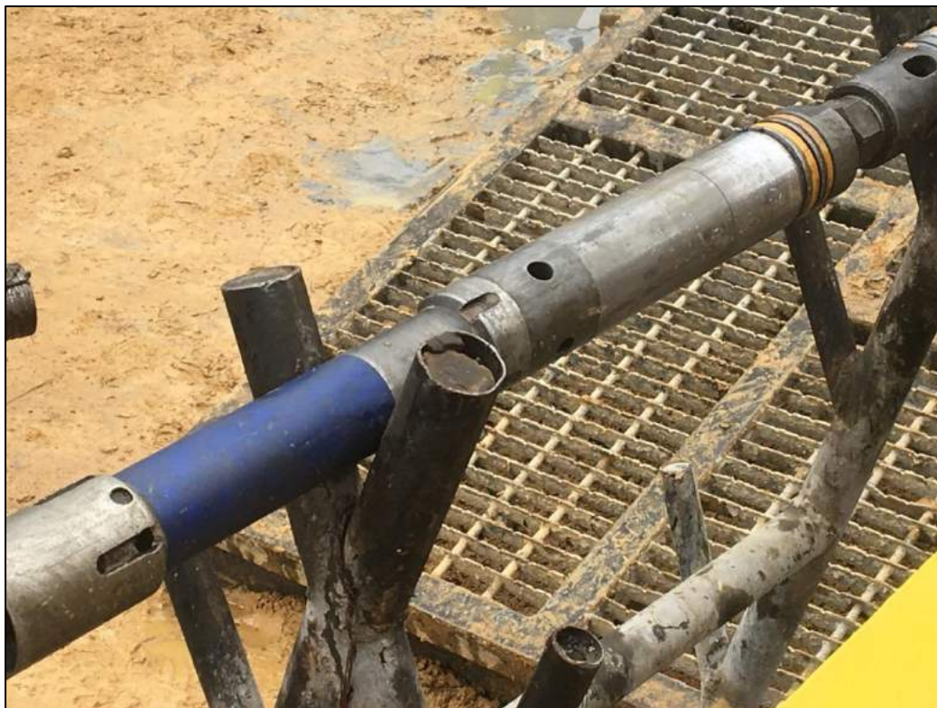
Figure 10-4: Devico downhole DeviGyro™ multishot survey equipment (source: Simon Mortimer, 2021).
